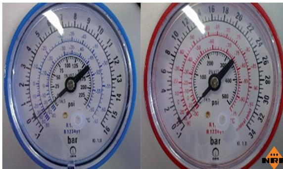
Photo 3 and 4. Low and high pressure gauge for R134a and R1234yf.
