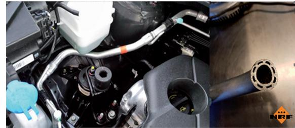
Photo 5. Internal heat exchanger for R1234yf refrigerant (photo: NRF)
