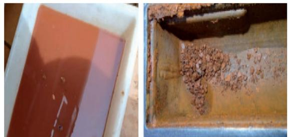
Picture 4. and 5. Sample of tap water used as coolant, and engine's corrosion. (NRF Photo)
