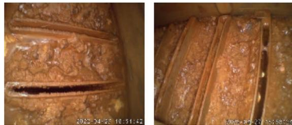
Picture 2. and 3. Rust sediments inside the radiator's tubes
